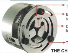
The size can be adjusted against the helical slot.
